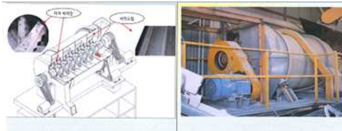
Bucket Aggregate Strike-peeling Equipment (Remove mortar stained on aggregate with striking impact and self crushing among aggregates)
